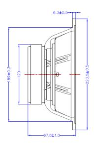
FS 33.0003 Hz **VAS** 65.1957 L RΕ 6.80 ohms **QMS** 2.239 **QES** 0.4086 **QTS** 0.3455 **SPL** 90.26dB 1m/2.83v SD 0.0206 m2 **CMS** 1.0990 mm/N MMS 21.1652 g **RMS** 1.9600 WM MMD 19.4903 g BL8.5460 L1kHz 0.2283 mH L10kHz 0.1151 mH X Max 9mm (1 way)
