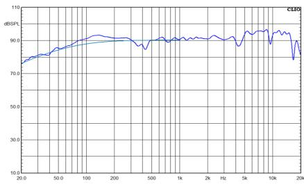
The frequency response above shows the measured anechoic axial sound pressure level using a standard IEC test baffle. Input 2.83v RMS, microphone distance 0.5m, SPL normalized to 1m value. The light blue line is the calculated low-frequency infinite baffle response from the parameters given in this datasheet. Impedance is measured in free space with a 1v input signal.
