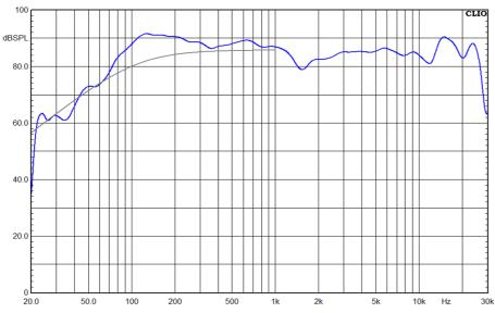
The frequency response above shows the measured anechoic axial sound pressure level using a standard IEC test baffle. Input 2.83v RMS, microphone distance 0.5m, SPL normalized to 1m value. The grey line is the calculated low-frequency infinite baffle response from the parameters given in this datasheet. Impedance is measured in free space with a 1v input signal.
